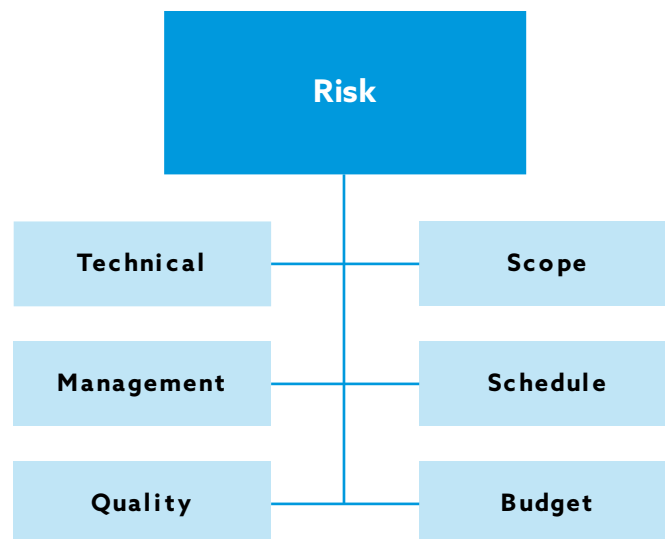
Figure III.2. Example of a risk breakdown structure
